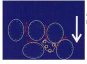
According to Stokes' Law the larger aggregates settle faster; as they do, they enmesh the uncharged protein particles.
